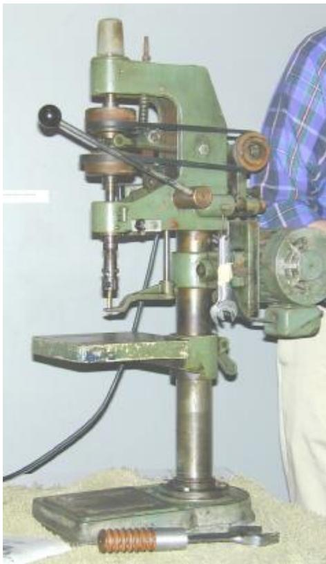
Joe Williams showed a tapping machine which uses two belts from the motor to the spindle. When pulling the lever down, one belt drives the spindle containing the tap in a forward direction. When pulled up, the second belt drives the spindle in a reverse direction, backing the tap out. Joe also brought an assortment of various types of tapes including spiral point and a thread milling cutter.
