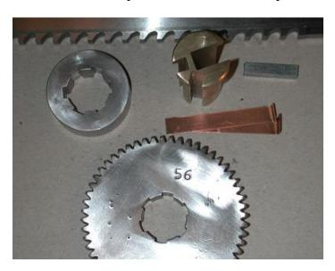
was slotted to fit the broach and the depth set to provide the depth of cut close to the required depth. It works out to cut one groove for the broach and two for an indexing key. The operation is to first broach one slot, rotate the pilot 180 degrees, insert a pilot key, and make another cut. Then rotate the broach pilot 45 degrees and insert the holding key and broach another slot. Continue until the hub has the six slots.
