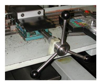
with a 1-1/2' Plastic Ball on the ends. They are set at about a 15 degree angle to the body to provide clearance for the operators hands.
