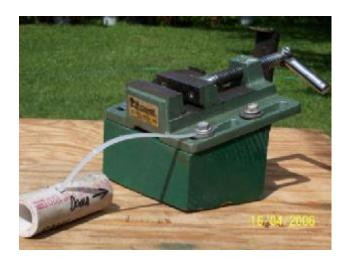
The first photo shows the front view of the saw with the vise mounted. Note that the automatic motor cutoff will not work, you have to flip the switch manually.
