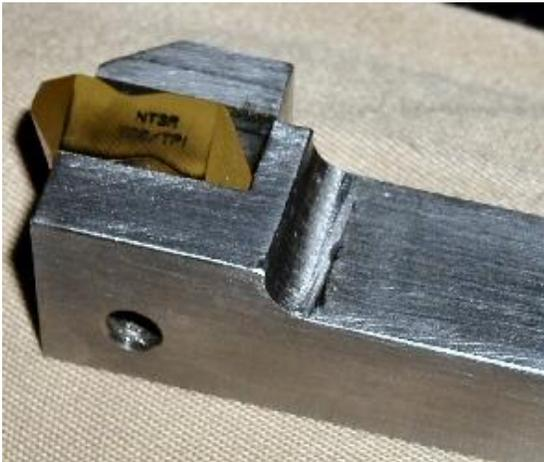
Ed Gladkiwski brought his index-able tool bit holder made from a 6-pointed wrench socket.
