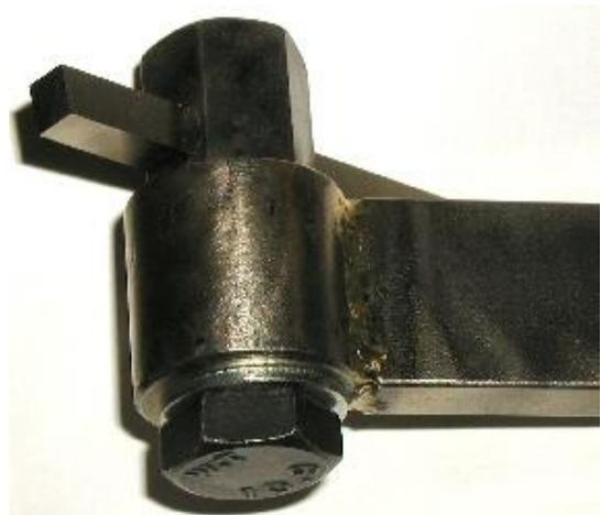
Dick Kostelnicek brought some large second hand drills where he converted the #4 Morris taper end to a 3/4 in. straight chuck-able end by turning in a lathe.
