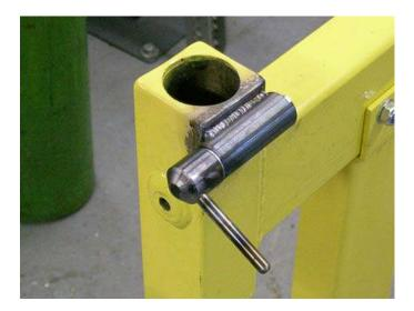
This photo shows the device welded in place. A 3-1/2" 3/16 bolt is used. The handle acts like a nut to tighten the device. Note that in this photo, the slit has not yet been sawed through the barrel and lower support.
