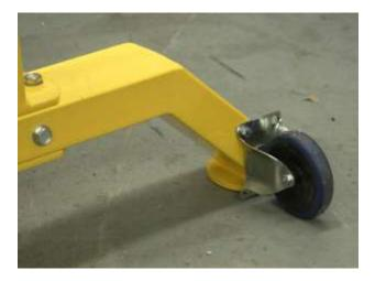
I installed simple 4" fixed casters to the front side of the front legs. To move the machine I just grab the top, tilt it forward, and away it goes! To secure
