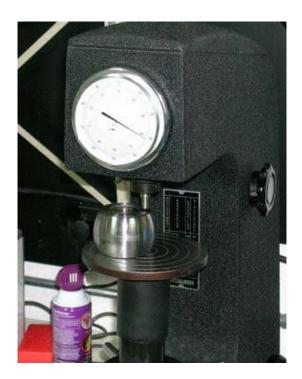
I was curious about the hardness of the rolls. Are they really made from heat treated alloy steel? I measured the hardness on my Rockwell hardness tested and found that both the upper anvil and lower read from 31 to 34 RC. This is what you would expect from prehardened 4130. I notice that most of the anvils available for sale are in this range, so I suspect the HF anvils will work just fine.
