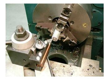
The end of the screw that touches the eccentric is unfinished. This uneven surface is a problem. So I faced mine off in a lathe and beveled the edges to help protect the threads. You don't need a lathe, a grinder or belt sander could be used to do the same thing.
