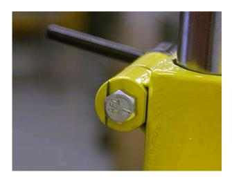
The photo above shows how the shoulder milled in the bar holds the bolt head and keeps it from turning.
