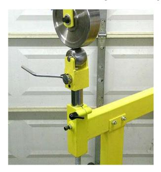
In this photo you can see the slit the was sawed. Tightening the handle securely locks the lower anvil support. Note that I replaced the old locking device with a cap screw and jam nut. The screw had to be machined into a dog point, just as the original had been. The handle used to tighten the lock was powder coated (more HF equipment).
