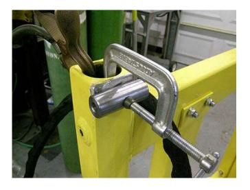
The photo above show the locking device ready for welding. It was made from a 2-1/2" length of 1" CRS. The rod was drilled through using a 13/32" drill. Then in the mill I flattened one side and cut a shoulder on the back end. This shoulder catches a hex flat or the retaining bolt. This allows me to adjust the position of the bolt so that the tightening handle is in a good position.
