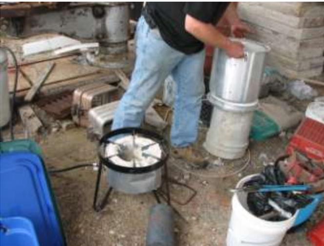
Light the fire, put in the crucible, then add ingots:
