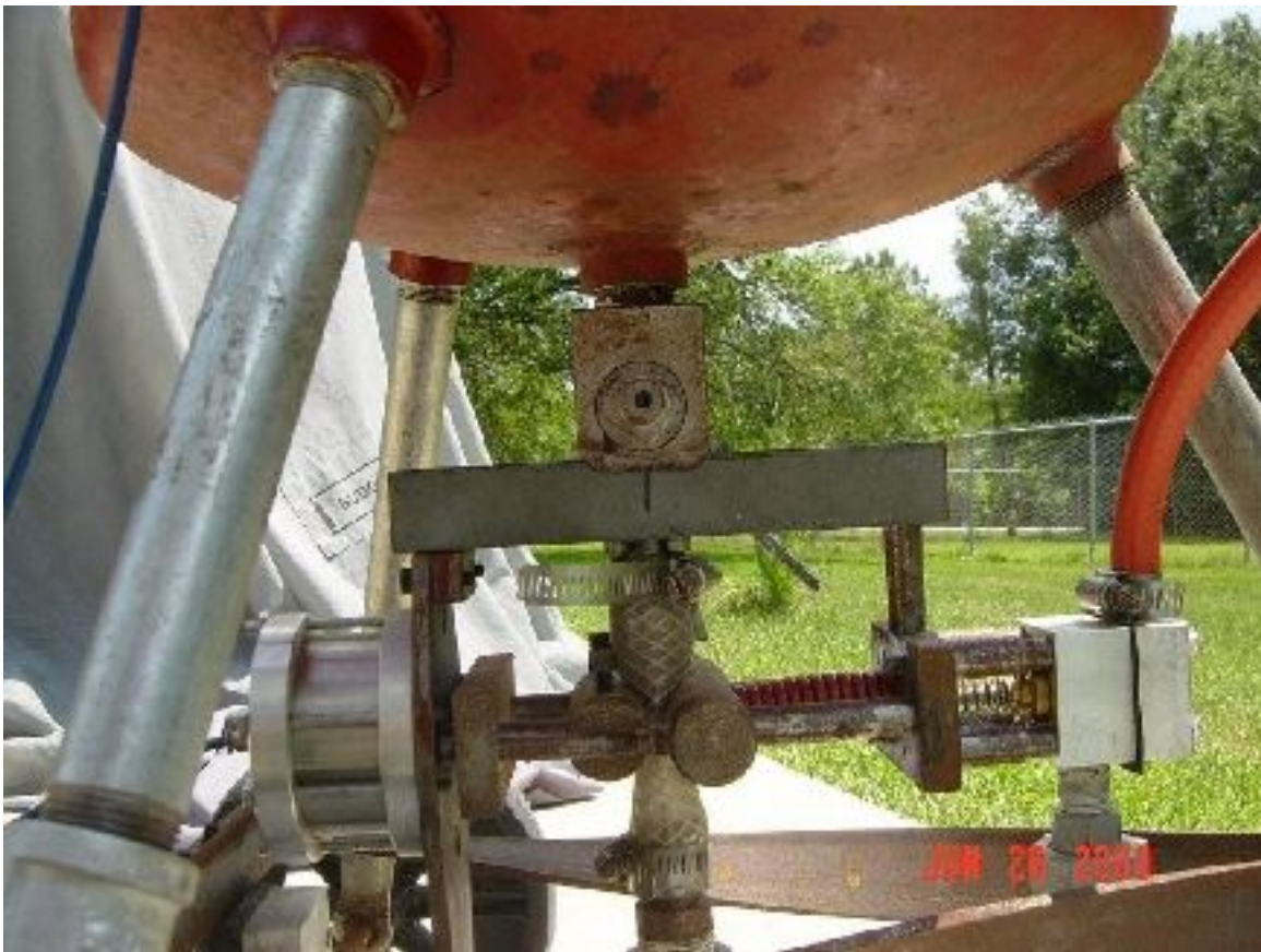
Figure 1. The control air cylinder is at the left, the jaw bars surrounding the vinyl sand hose in the center, and the main air supply valve on the right.
