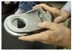
Shannon DeWolfe showed a wedge filter (left photo) that is part of an X-ray machine, and allows organs such as the lungs to be shaded while X-raying the heart.
