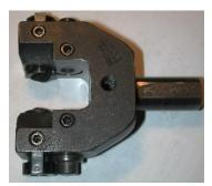
It's a B&S Mfg. Co. number 185-220. The straight knurls (right photo) can be set at any angle and adjusted to accommodate a range of stock diameters. The tool is designed to be held in a turret tool holder and has a 3/4" diameter shank. During the knurling operation, It approaches the work along the turning axis. Standard lathe knurling tools
