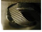
approach the work in a radial direction, either with single or double knurls. These are pressure formed knurls.
