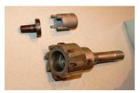
Dick Kostelnicek has a face mill cutter with a negative rake. He had difficulty tightening the bolt that secures the cutter head to a R8 arbor. Dick made a tool having four silver soldered projections on an annealed hex nut socket to facilitate tightening securing bolt (left photo).
