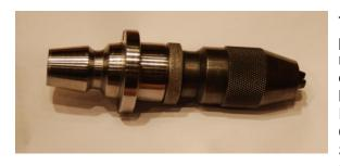
The second project was making three quick-connect tool holders for the Royal Quick-Change Tool System on his mill. The
