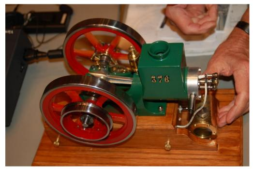
Alan May brought in his model engine called the 'Farm Boy Hit and Miss 4-Cycle Engine' designed by www.jerryhowell.com. This little engine runs on acetone, and Alan built it from the model plans. Alan spared no detail, as one can see from the picture. The engine is designed to use an 'O' ring on the piston instead of normal cast iron piston rings. Without a load, the Farm Boy will turn between 20 to 30 revolutions between Hit and Miss firings.
