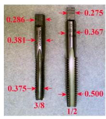
Jacobs chuck will drive them without having being tightened excessively. Also, any of the drivers can be grabbed by a ½-inch round collet. Make sure that when you mill the side opening in the driver that the slot is the correct width and depth in order to engage three sides of the square drive tang on the tap. Have the appropriate tap handy to check the fit as you mill
