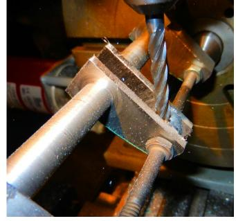
dimension. I made the cut starting in the middle of the 3/8-inch gap, and worked out to each side. I experienced two problems while making this cut
