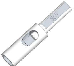
I made tap drivers for my larger taps; viz., 1/2, 7/16, 5/8, and 3/4-inch diameter (see left drawing). The shanks of the drivers are all ½-inch diameter with three 120-degree spaced flats. This ensures that a 3-jaw
