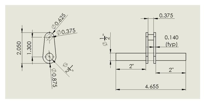
Above is a drawing of the crankshaft. I rough machined the crankshaft stock on the mill, and turned the main  $\frac{1}{2}$ " shafts on the lathe. But then, I had a problem. The gap available for a tool to machine the smaller  $\frac{3}{8}$ " shaft is only  $\frac{3}{8}$ "; not much wider than the  $\frac{1}{4}$ " gap of the crankshaft for the engine in the earlier article. But this crankshaft has a 1.3" throw, almost twice the  $\frac{3}{4}$ " throw of the other crankshaft.
