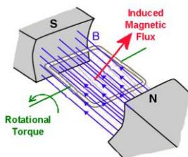
Club member *Dick Kostelnicek* gave a presentation on 'AC Induction Motors'. You can view his presentation slides at [this web link](#). He began by describing the two types of excitation for stators commonly found on all electric induction motors. A motor with a DC excited stator may have either a permanent magnet built into the rotor or use a commutator for the electrical coupling to
