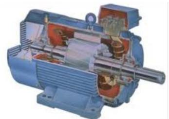
the rotor. On the other hand, an AC excited stator relies on magnetic induction for electrical coupling to the rotor. The AC induction motor was the primary focus of Dick's talk.
