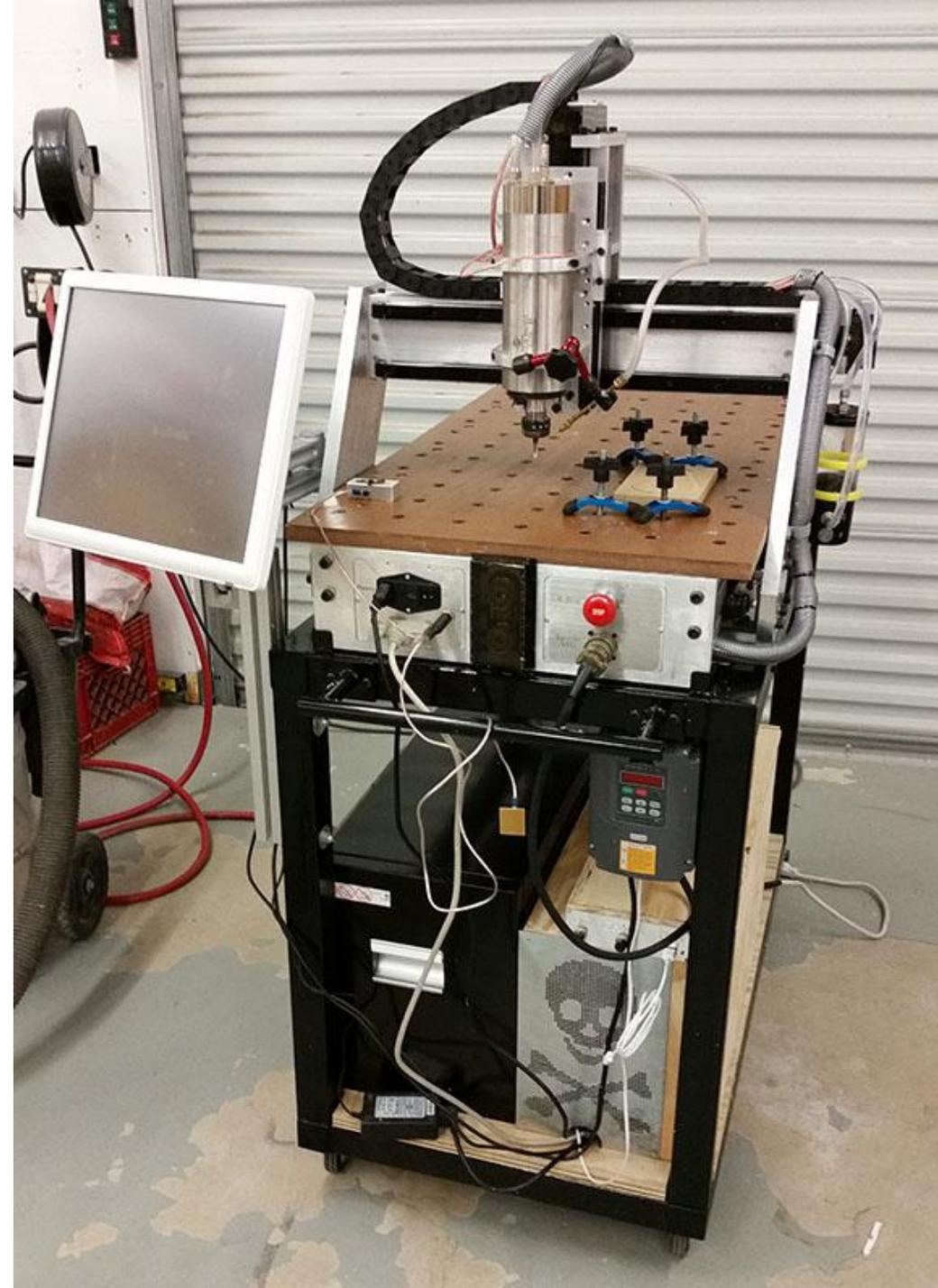
The machine I brought today is a modified Chinese 2030 type machine. This machine was design specifically for milling printed circuit boards and other thin flat work.
