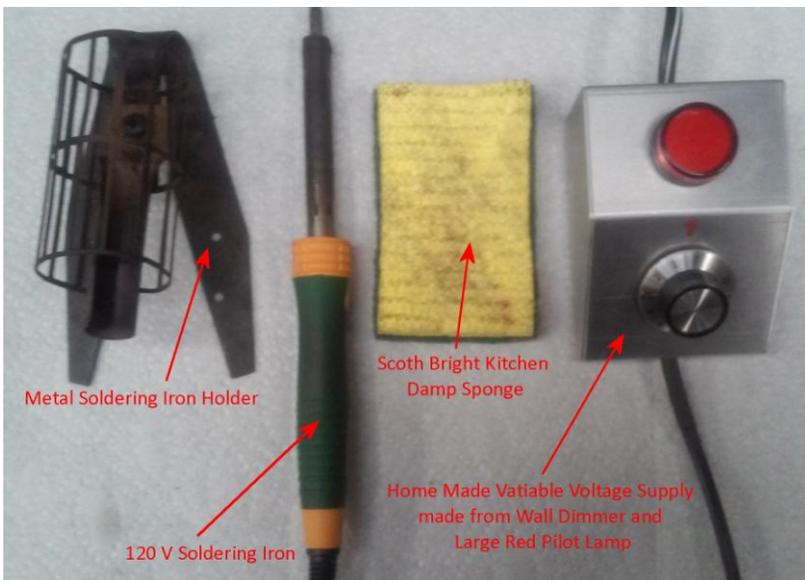
I'm shocked at the price of just a mediocre soldering station for fine electronic work at \$75 or more. So, I made a station from common stuff lying around my home and shop.
