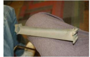
*Paul McKneely* showed a bracket made of injectable polyethylene plastic using the injection molding process (right photo). Following the theme of today's presentation, Paul discussed film making with virtual sets and the use of programmable controllers for programmable lights.
