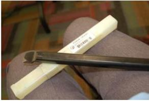
*Richard Douglas* shared with the club a good source of metal stock, M&M Metals. He also exhibited a turbine vane that had been removed from service (right photo) and a 1" diameter by 12" long boring bar (left photo).
