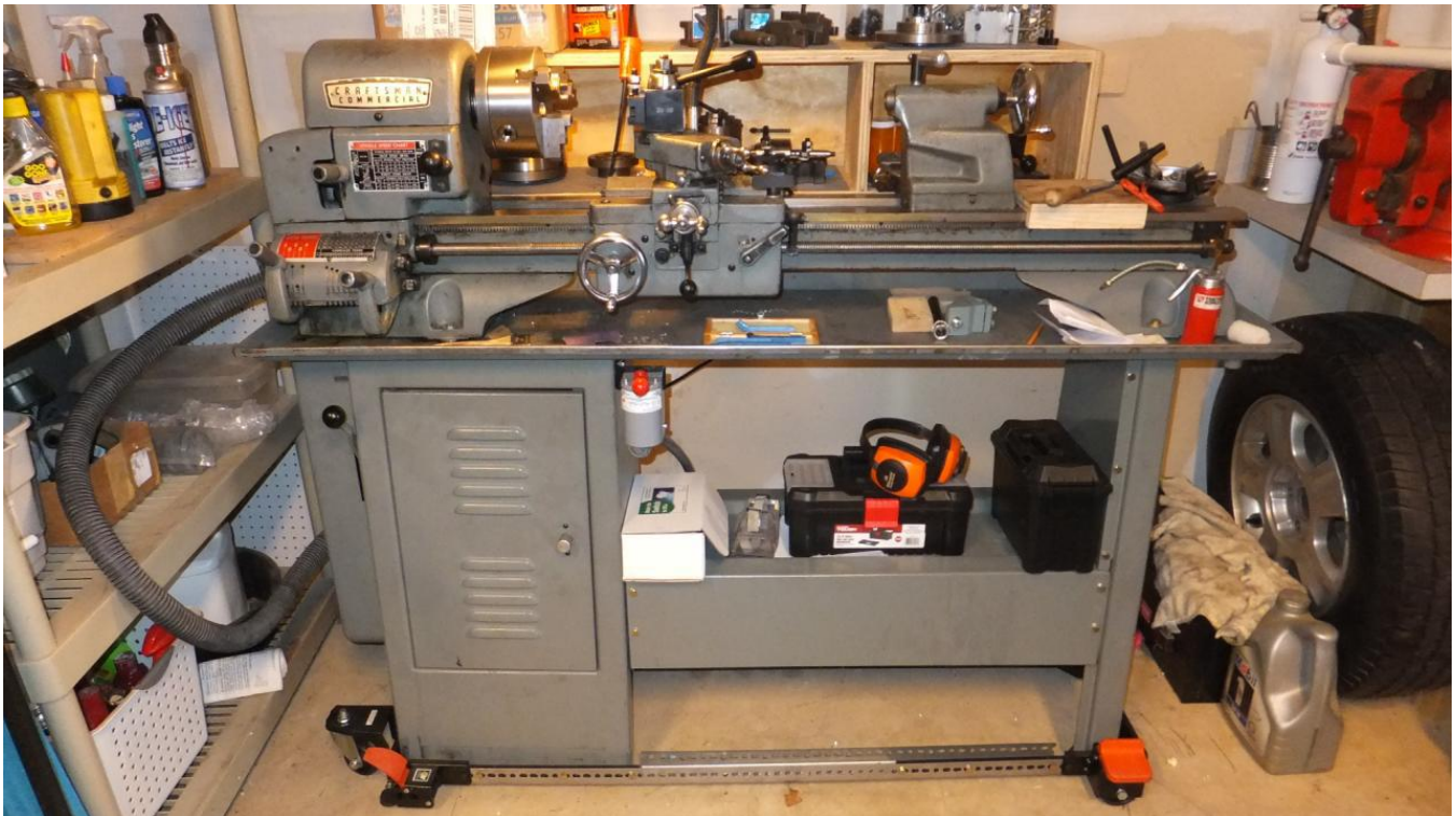
This photo is of my refurbished 12-inch Craftsman lathe mounted on a mobile base in my garage.
