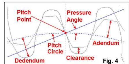
When two gears are in mesh, the tooth crests of one gear plunge into the throats of the other. The depth that they reach beneath the pitch circle is the addendum of the plunging tooth. Hence, the working depth **WD** of the teeth is twice the addendum:
