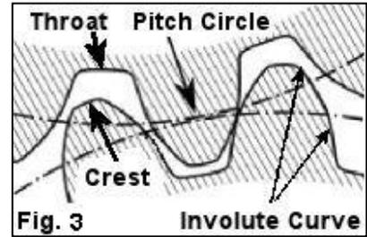
rotational speed ratio as their gears. The tooth size is specified by its circular pitch **CP**, the tooth-to-tooth distance along the pitch circle. Larger **CP** means bigger teeth. The diameter **D** of a pitch circle having **N** teeth is:
