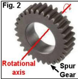
A spur gear's shape doesn't vary along the direction of its rotational axis (Fig. 2). Modern gear teeth have an involute curve profile (Fig. 3). Each tooth has a crest and throat. The pitch circle is an imaginary curve passing through each tooth close to 1/2 its height. Pitch circles represent the surfaces of two wheels in non-slip contact that will produce the same
