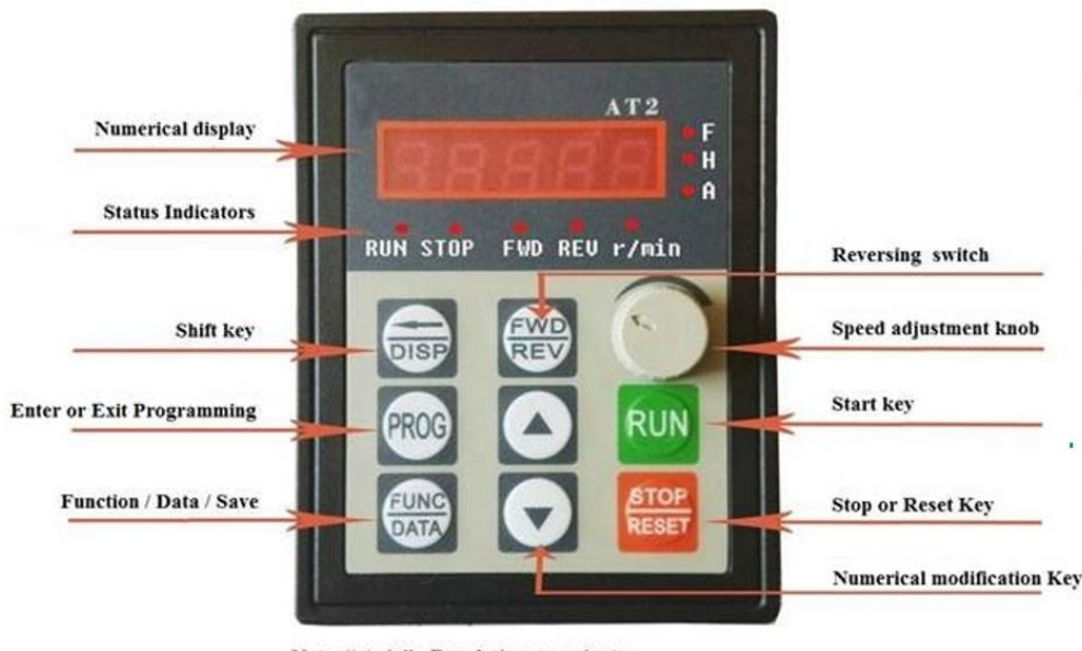
Figure 1. Front of VFD
