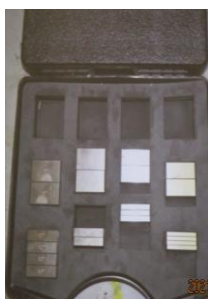
Illustration 6: Metal shims with magnets
