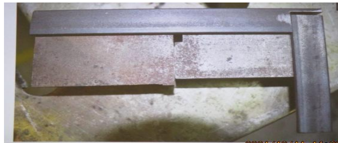
Illustration 2: Alternative to 45 degree joint
