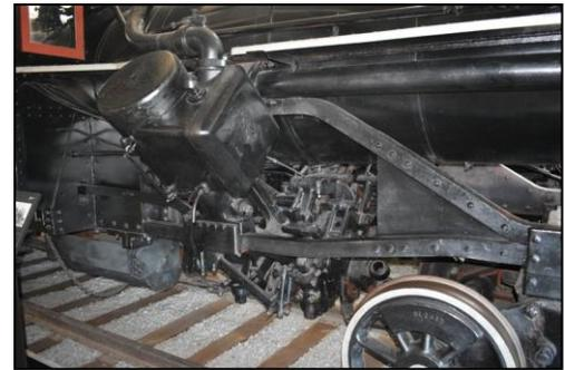
Photo 20: Close-Up of Twin Vee Steam Engine
