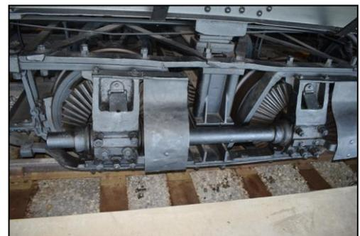
Photo 22: Bevel Gears on Shay Locomotive
