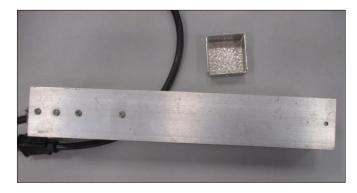
*Mark Heidorn* showed a heater he made to protect his citrus tree during cold weather. The heater is made from 2x2 aluminum tubing and two 100 watt resistors. The tubing serves as a heat sink for the resistors that are powered by 120 vac. Once the six foot tall tree is covered with a tarp, the heater is placed on the ground near the tree and under the tarp. The radiant heat produced is sufficient to warm the tree when the outside temperature falls to 25 degrees Fahrenheit. See photo at left.
