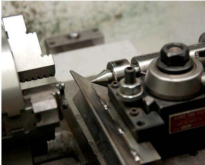
Find a cutting device that is very close to the diameter of the tube your part will mate up with. Mine was easy. Since it was 0.750" mechanical tubing, I used a 3/4" endmill. Be careful when mounting tools such as endmills in your chuck. Endmill shanks are very hard, and can damage your chuck jaws. Other tools you could use are holesaws and boring heads. Roughing endmills are generally used in the high-dollar commercial tube notching machines.
