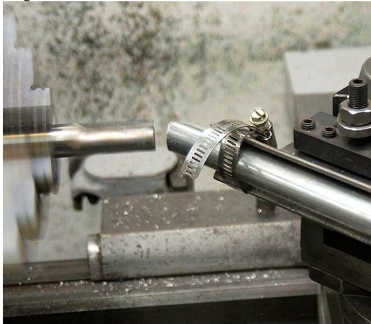
As you can see in the photos, my clamping technique was on the low-cost side. Hose clamps work good on Aluminum, but for steel, I think that a stronger clamp such a “U” bolts would work better.
