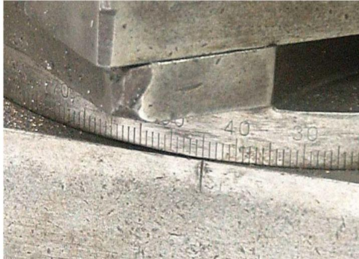
The desired angle of cut is set using the compound. For this cut, the compound was set for a 45-degree angle.
