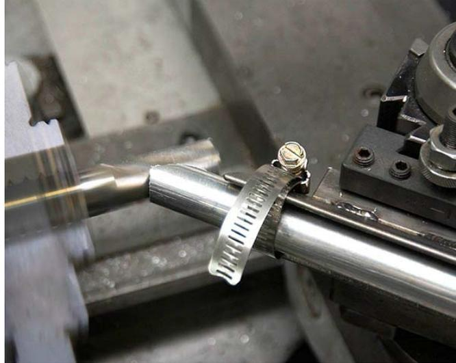
I was cutting soft aluminum with only a 0.025" wall, so my biggest concern was that I didn't crimp or bend the end of the tube. So I made fairly light cuts. If you're cutting 4130 tubing, remember to slow down the cut and use some type of coolant.
