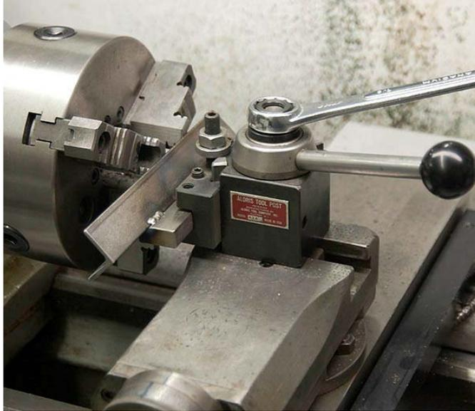
Two adjustments must be made when mounting the jig on the toolpost. First, set the compound to zero degrees, lock the jig in a toolholder, then square the toolholder with the face of the lathe chuck by rotating the toolpost. The next adjustment is to set the height of the jig. It is important that the center of the V be aligned with the lathe centerline. I used a center in the tailstock to bring it close, then tweaked it in using some test cuts. Once set, it should remain accurate.
