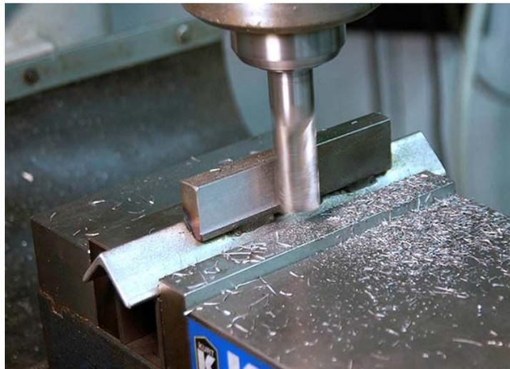
After the weld cools, put the assembly back in the mill and take a light cut along the bottom of the block of steel. This is to assure that the center axis of the V-Block is aligned with the ways of the crossfeed and the jig is level.
