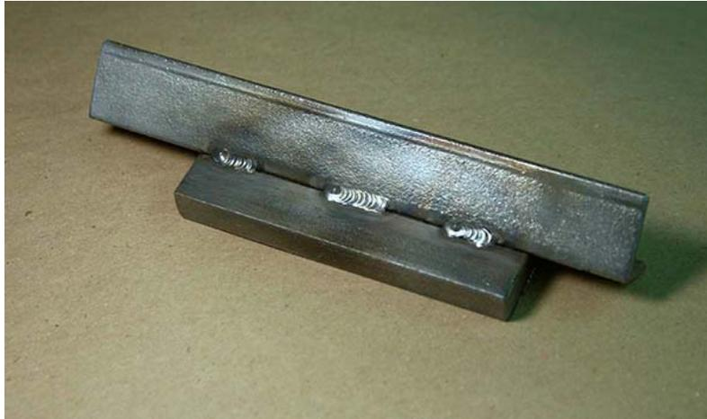
The two pieces are carefully positioned on the welding table and welded together with an intermittent bead. A continuous bead may cause warping, so don't get too carried away with the welding.
