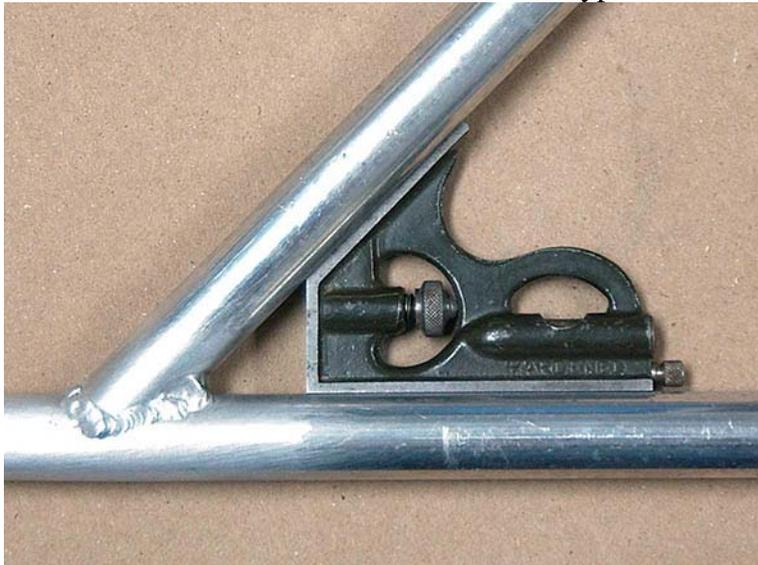
Here's the result. A very tight and accurate joint and an accurate angle (ignore the welding job, that 0.025" wall tubing is tough to work with).
