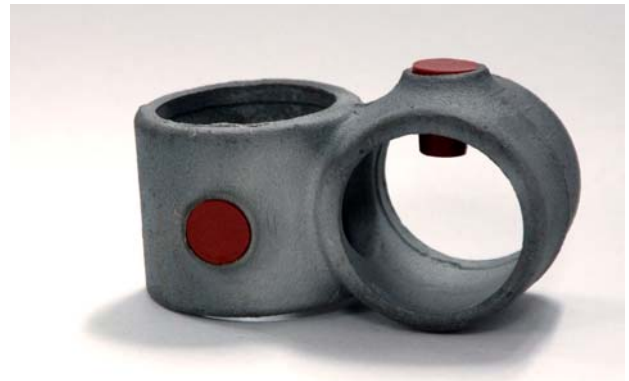
The part has been cleaned and plugs inserted to protect threads
