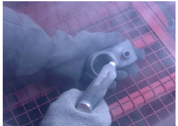
Sandblasting with Aluminum Oxide grit
