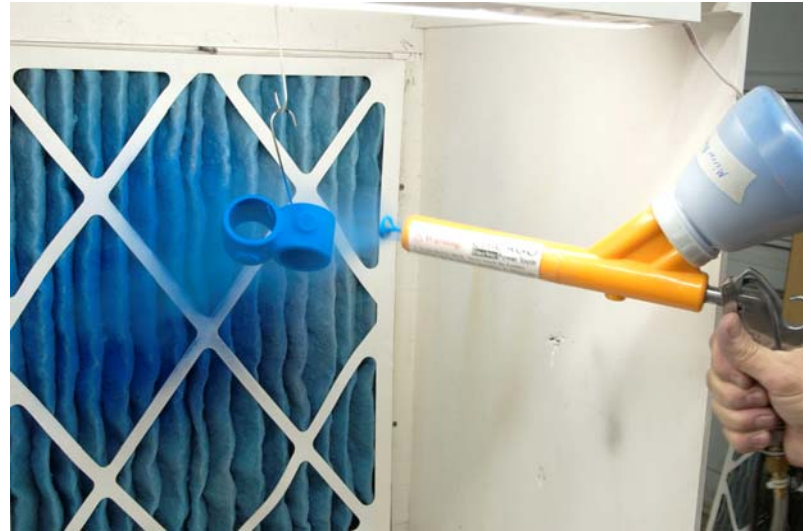
The electrostatic charge makes the powder stick to the part.
