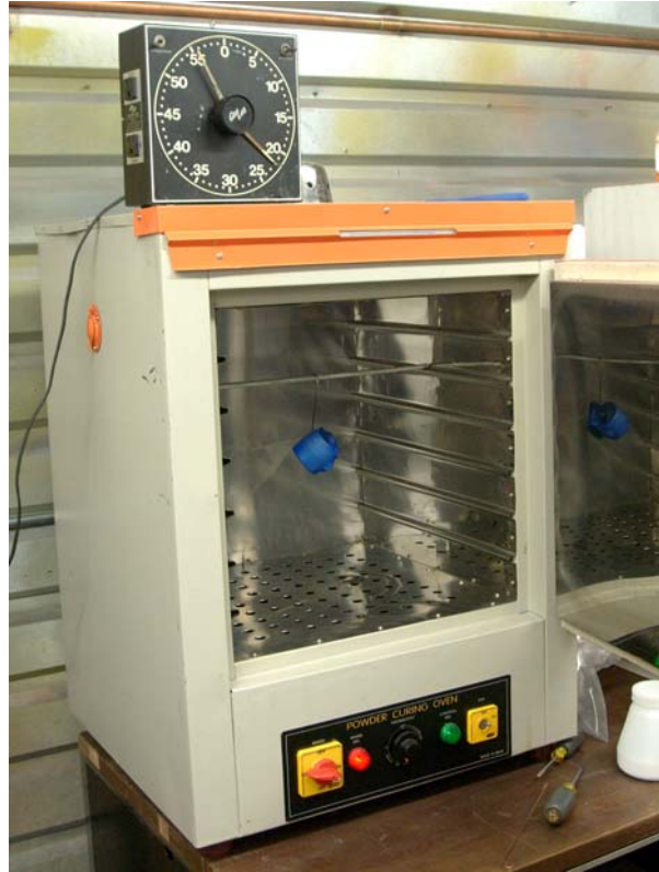
The part is in the oven for curing
